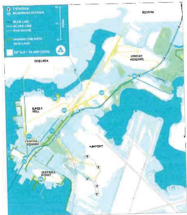
Toole Design created this map for the Plan East Boston multimodal transportation network overlaid with a flooding scenario with 36" of sea-level rise (predicted for 2070) and a 100-year storm at high tide.
